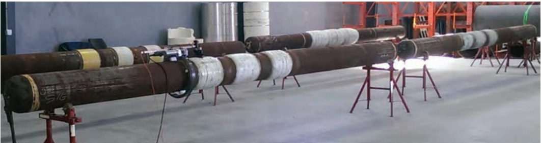
Pipeline repair test samples containing simulated defects/anomalies.
