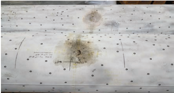
Mechanical Damage samples to be used for ILI performance Testing.
