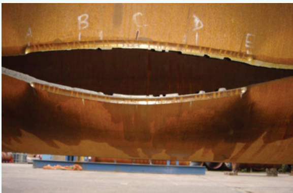
Test 2 Vessel After Rupture.
