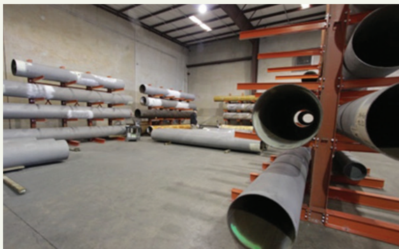
Former in-service pipeline samples with surface preparation completed and ready for inspection.
