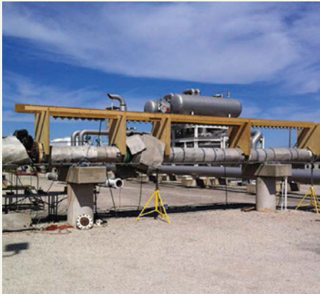
Figure 1 An assessment of how heat transfer effects at low flow rates impact the flow measurement accuracy of ultrasonic meters at low flow rates.
