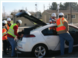
Gas sensor and related equipment installed in an automobile for ground-based monitoring and surveillance of pipelines.
