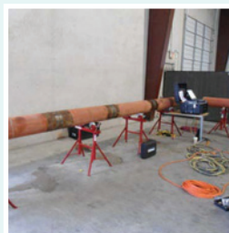
Test specimen at NDE Repository undergoing inspection study for detection and sizing of fatigue cracks in girth welds
