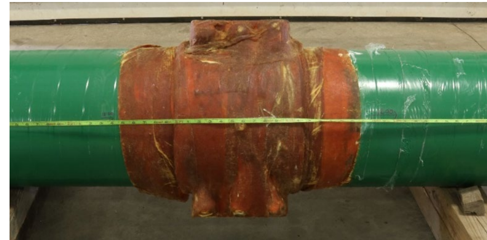
Backing strip behind longitudinal seam of over-sleeve
