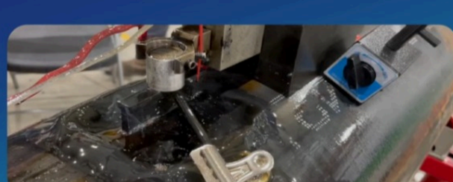
EDM notching of corrosion features coincident with long seam
