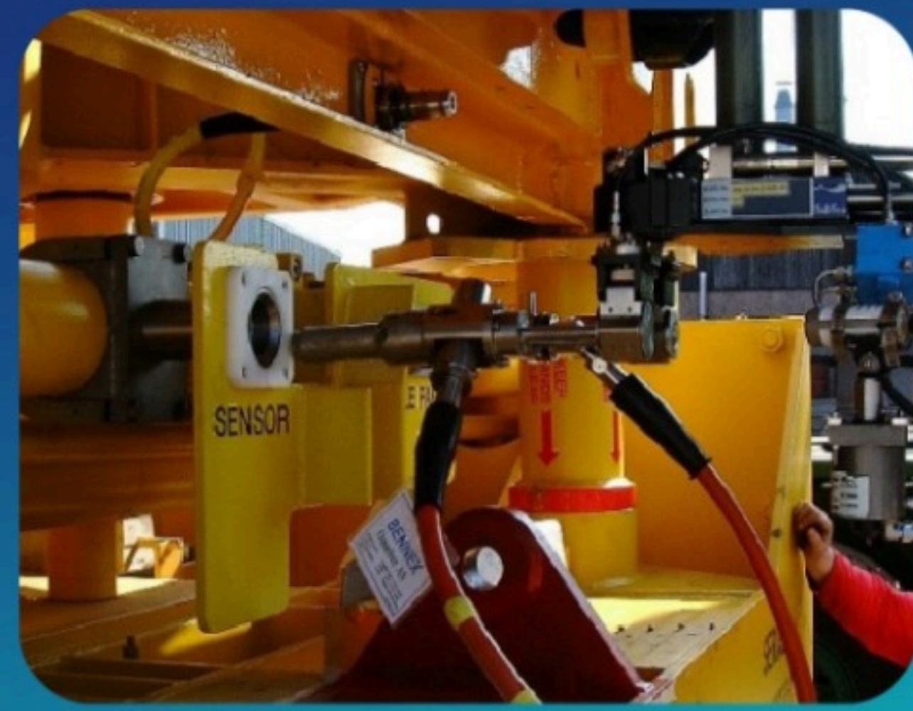
Installation of a subsea sand detector
