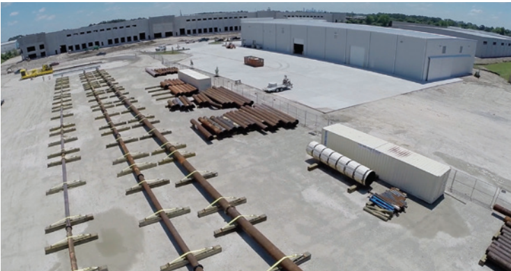
State-of-the-art pull test facility with 24, 16, and 12 inch pull test strings.
