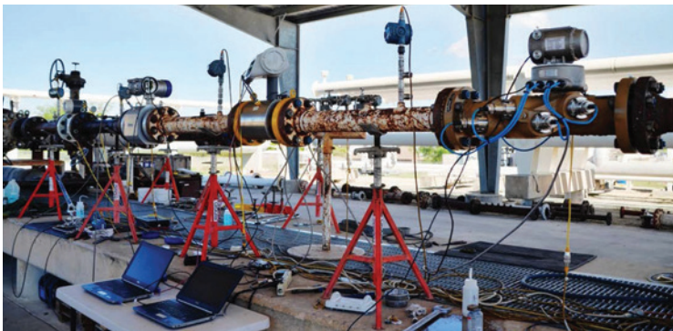
FIGURE 7 Test setup of ultrasonic meters in liquid transients. Meters from four different manufacturers were evaluated.
