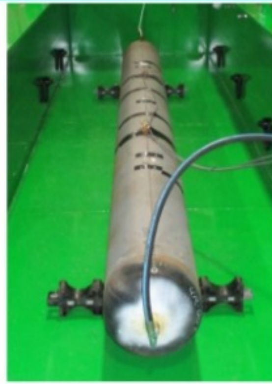
Unrepaired Sample in a pressure testing chamber for MATR-3-13 Project Evaluating Installation Techniques for Pipeline Repair Methods
