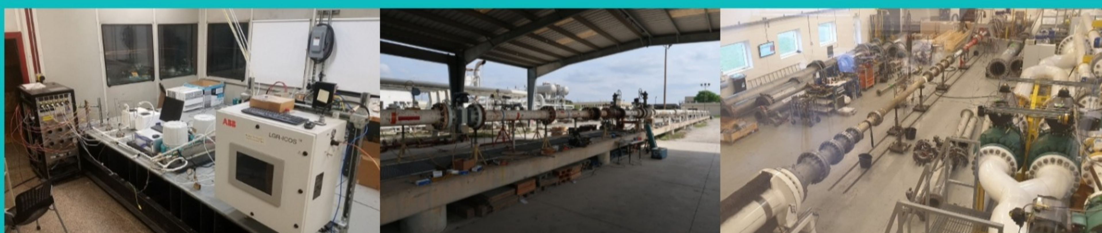
PR-015-19606-R01 in-situ USM flow verification testing setup at the Southwest Research Institute Metering Research Facility.
