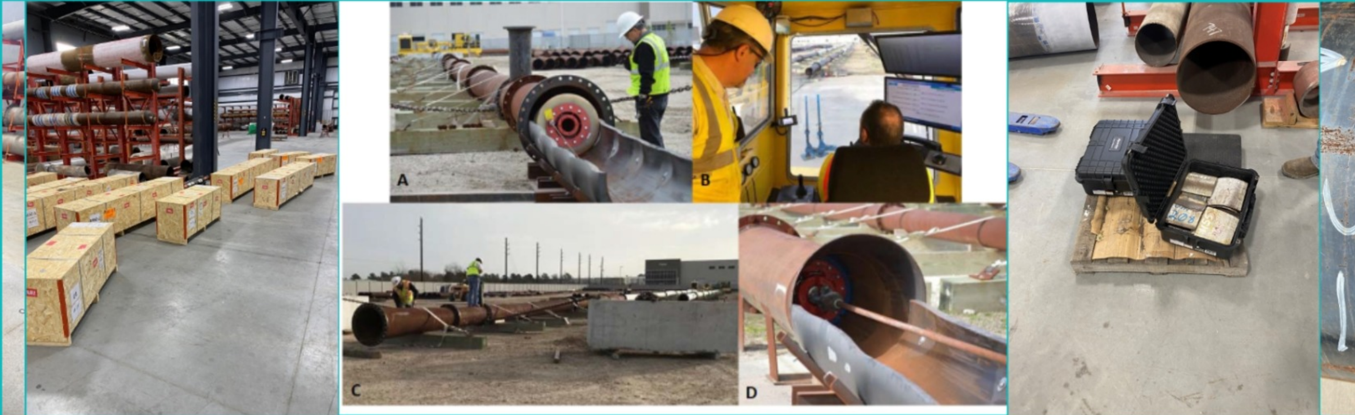
The 24" mechanical damage ILI project was based on the results of many pull tests.
