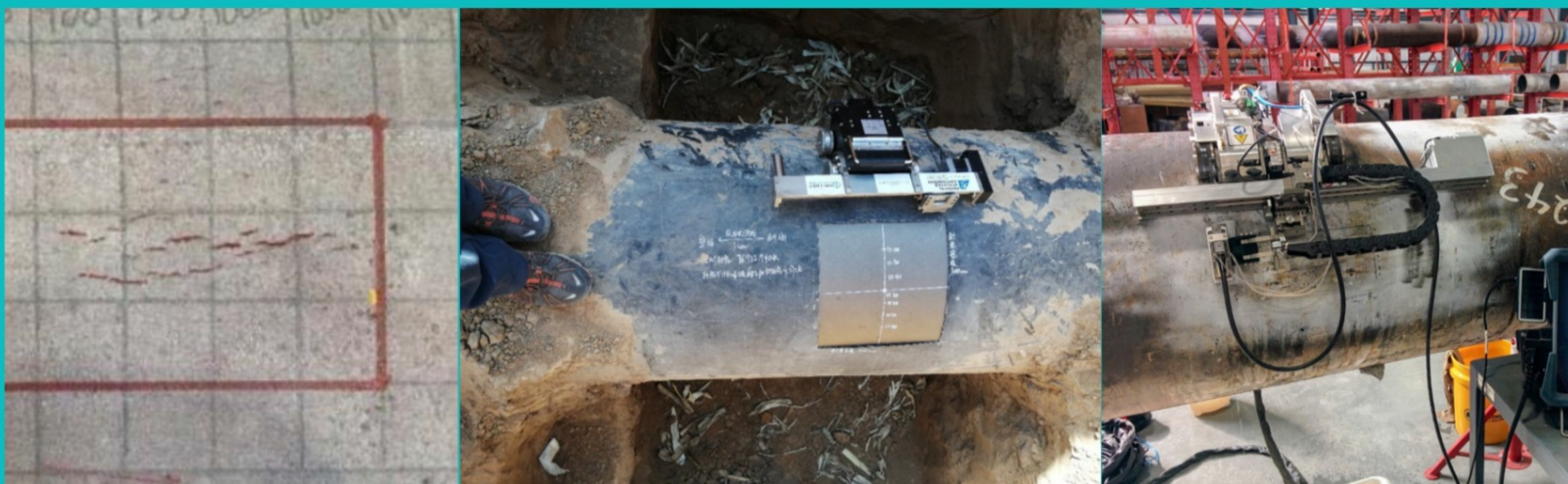
For NDE-19: A dig site in China where in-ditch NDE is being used to assess I&I performance for detecting and sizing pinholes.
